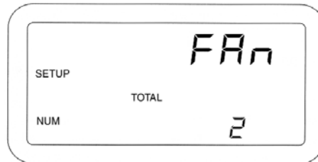
Figure 22 Fan Speed Sensor Display
