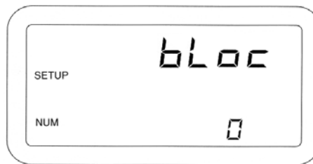
Figure 35 Blockage Mode Display
